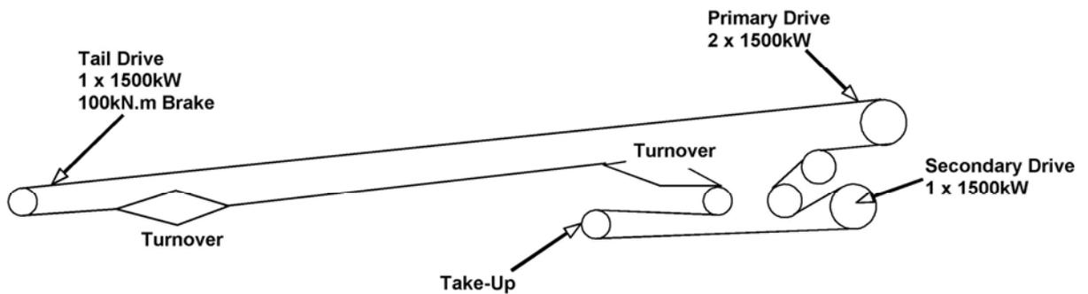
**Figure 2. Layout of Tianjin Coal Transport Conveyor**
