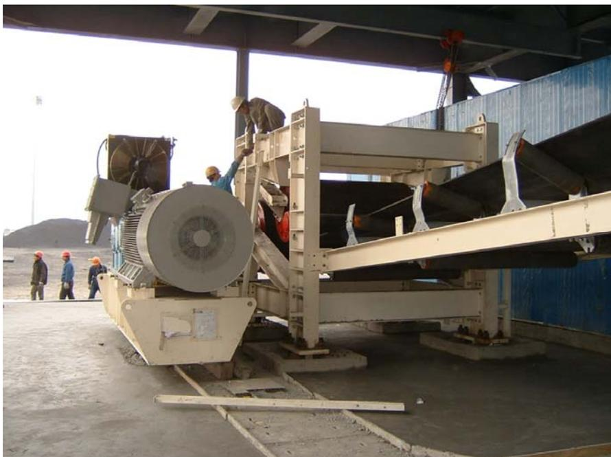
**Figure 3. Tianjin Coal Conveyor Tail Drive**
