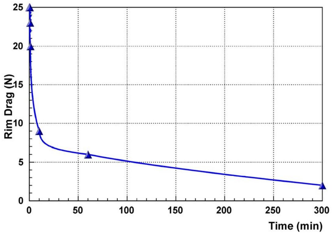
Figure 4. Tianjin Coal Conveyor – Carry Roll Rim Drag Measurements
